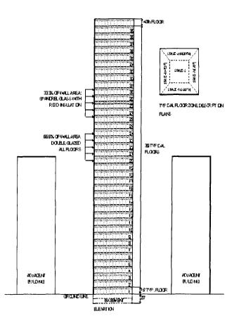
Figure 3. Three Dimensional Model of Prototype Building The figure, shows the spatial relationship of the prototype building and its surrounding buildings. Based on visual analysis of photographs of the selected sites, all buildings are 100' x 100' in length and width. The surrounding buildings are 20 stories tall. The middle building is 40 stories tall.
